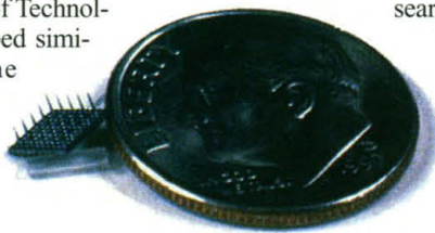
Brain bug. Several teams use this 25-electrode array (4.2 mm 2 ), seen next to a dime, to record neural signals from a monkey's cerebral cortex.
