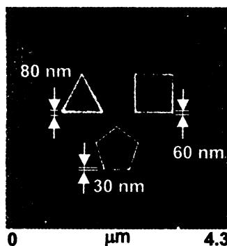
**Fig. 4.** SAMs in the shapes of polygons drawn by DPN with MHA on an amorphous Au surface. An ODT SAM has been overwritten around the polygons.
