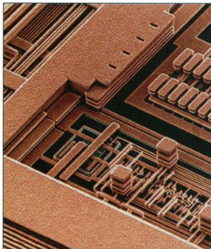
**Complex wiring on a small scale.** Top-down view of an IBM seventh generation microchip. The silicon dioxide insulating layers have been selectively removed to reveal the complexity of the wiring schemes.
