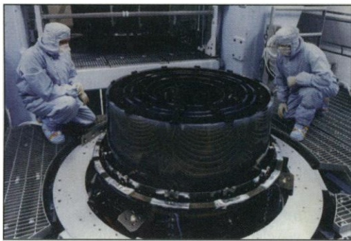
The fairest mirrors. Chandra's concentric quartz mirrors, which focus x-rays that graze their surfaces.
