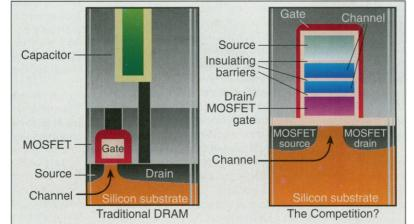
**Packing more punch.** A new design for a working memory chip (right), featuring transistors posing as capacitors, could potentially shrink memory chips and make computers boot up and run faster.
