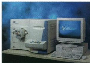
The Finnigan LCQ DECA includes unique data reduction tools for managing and interpreting multi-stage MS/MS data.
