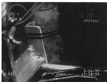
Fig. 3. Mass of flocculant \text{CO}_2 hydrate created at a 905-m depth, T = 4^\circ\text{C} , by vigorous injection of liquid \text{CO}_2 through a small-bore tube. The pure hydrate density is greater than that of seawater but at the time of formation in this manner occluded liquid \text{CO}_2 and trapped water warmed by the heat of formation create a buoyant mass.
