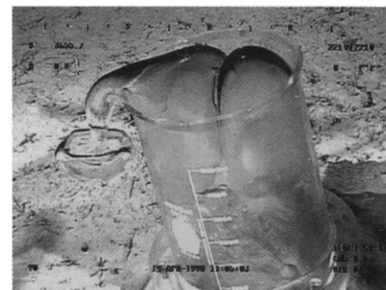
Fig. 5. Overflow of liquid \text{CO}_2 from the 4-liter beaker onto the sea floor at a 3650-m depth. A mass of transparent hydrate ( \text{CO}_2 \cdot 5.75\text{H}_2\text{O} ), formed at the upper interface, sank to the bottom of the beaker and pushed out the remaining liquid \text{CO}_2 . Ejected liquid \text{CO}_2 was highly mobile and did not appear to penetrate, or interact with, the sediments.
