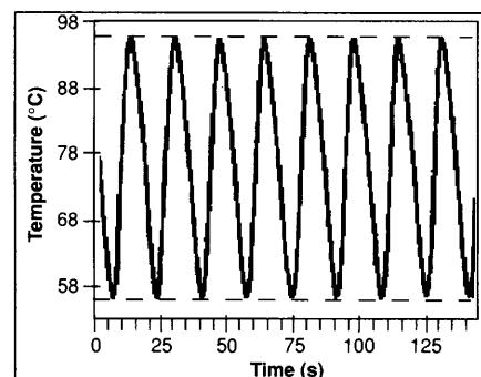
**Fig. 3.** Temperature profile of a reaction performed with a 17-s cycle time. A thermocouple connected to a strip-chart recorder was placed in a reaction tube in a chamber during thermal cycling. The dotted lines indicate the set temperatures of 96° and 56°C. Although the set time at each temperature was 1 s, the actual time that the solution was at each set temperature was less than 1 s because of the lag in heat transfer from the silicon chamber walls to the solution in the plastic tube.
