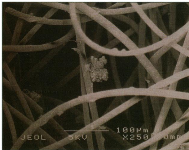
Web site for cells. The micrograph shows smooth muscle cells growing in a porous polymer used for tissue engineering.
