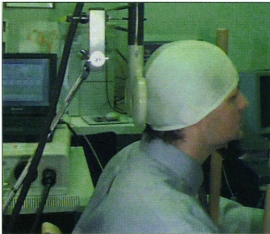
Brain zapper. This TMS device focuses a magnetic field that disrupts specific brain areas.
