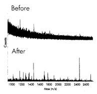
In-gel digestion of "spot 223" of 2D gel before and after ZipTip<sub>C18</sub>
