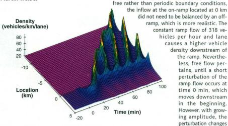
its propagation speed, reverses its direction, and finally induces another, bigger perturbation, when passing the ramp. This process repeats again and again, in this way generating the oscillating RH state. When passing the ramp, the perturbations continue their way upstream, until they merge with one of the humps that were born later.
