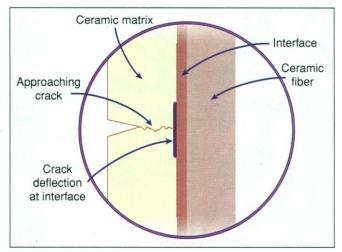
**Fracture stopper.** Cracks that initiate in the brittle ceramic matrix encounter the interface material separating the fiber from the matrix. In a tough ceramic composite, the matrix crack is deflected at the interface and ceases to propagate, allowing the composite to continue functioning in a structural sense.
