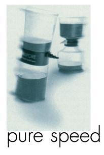
Filter in half the time with the Stericup™ vacuum filter unit. Our patented fast-flow, low proteinbinding Millipore Express™ membrane gives you faster filtration with bacterial retention. Features include a unique no-tip, easy-grip design; a recessed bottom that allows stacking for convenient storage; and a tab inside the funnel that holds a prefilter securely in place.
