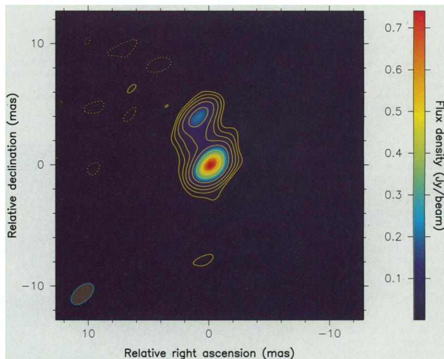
**Fig. 3.** A 1.6-GHz image of the quasar 1548+056 made from an observation with HALCA (using the Goldstone and Usuda tracking stations) and from telescopes in Australia, China, and Japan. The synthesized beam is 2.3 mas by 1.3 mas (FWHM) at a position angle of  $-48.2^\circ$ . The residual noise level in the image is 3.6 mJy per beam (rms). The contours are at  $-1, 1, 2, 4, 8, 16, 32,$  and  $64$  times 9 mJy per beam. At the distance of the quasar, 1 mas corresponds to 18.6 light-years.
