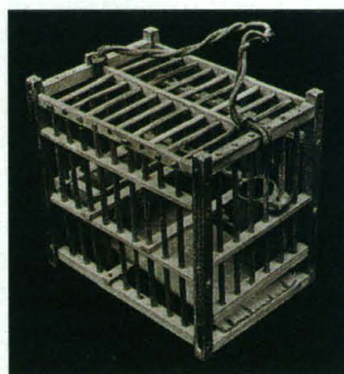
Soul sacrifice. Canary's cage used to detect the release of toxic gases in a mine. The death of the canary serves as a warning that toxic gases are present. (Below) A canary cage in use.
