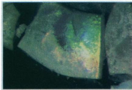
**Fig. 1.** Photograph of crystals of air spheres in  $\text{TiO}_2$ . The crystals were made from templates consisting of particles with radii of 225 nm. The width of the field of view is 0.5 mm. The bright blue and green reflections are optical Bragg reflections from the crystals. Several colors appear because the angle of incidence of the illuminating white beam varies with respect to the crystal planes.
