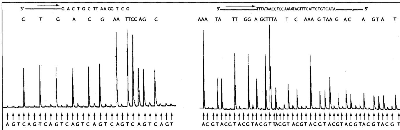
**Fig. 2.** Pyrosequencing was performed on a 35-base-long oligonucleotide template (Left) and a 130-base-long PCR product (Right). About 2 pmol of the template-primer was used in the assay. The reaction was started
