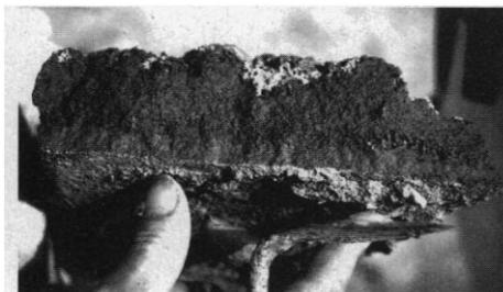
**Fig. 2.** Section (~30 cm by 8 cm) across slab of synthetic basalt. (Photo: Paul Zimansky)
