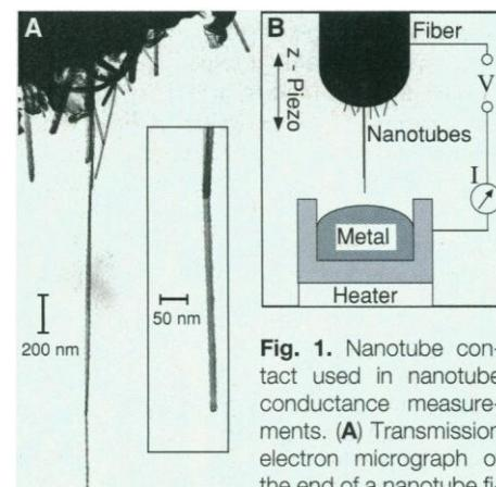
**Fig. 1.** Nanotube contact used in nanotube conductance measurements. (A) Transmission electron micrograph of the end of a nanotube fiber recovered from the
