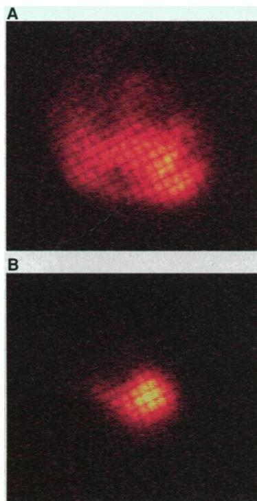
**Fig. 4.** Soft x-ray output beam for harmonic orders 23 through 31: (A) unphase-matched, detector set to high gain, and (B) phase-matched, detector set to low gain.
