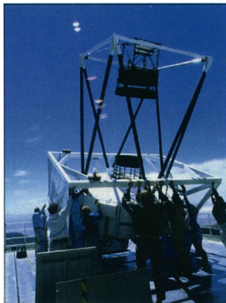
Aiming high. Sloan Survey members point the 2.5-meter telescope to the zenith after mounting the electronic camera.
