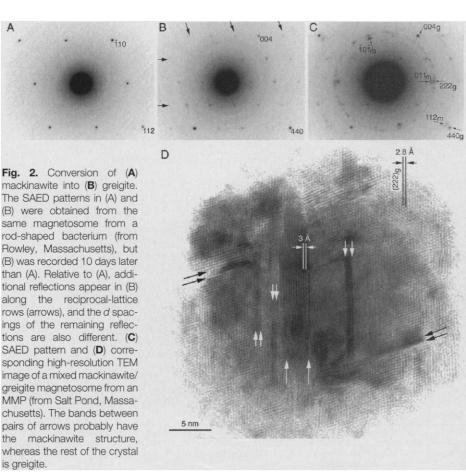
tures can occur with the S array preserved, except for a slight contraction of the S substructure as indicated by the spacings of adjacent close-packed layers, which decrease in the sequence cubic FeS  $(d_{111} =$  $3.12 \text{ Å}) \rightarrow$  mackinawite  $(d_{101} = 2.97 \text{ Å}) \rightarrow$ greigite  $(d_{222} = 2.85 \text{ Å})$ .
