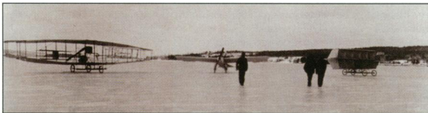
Early flying machines. Three of the last planes designed by Bell and his associates, on the frozen Bras d'Or Lakes, Nova Scotia, in early 1910: the biplane Baddeck 1 , the Hubbard monoplane, and Bell's own Oionos , his final attempt at using a tetrahedral design for powered flight.
