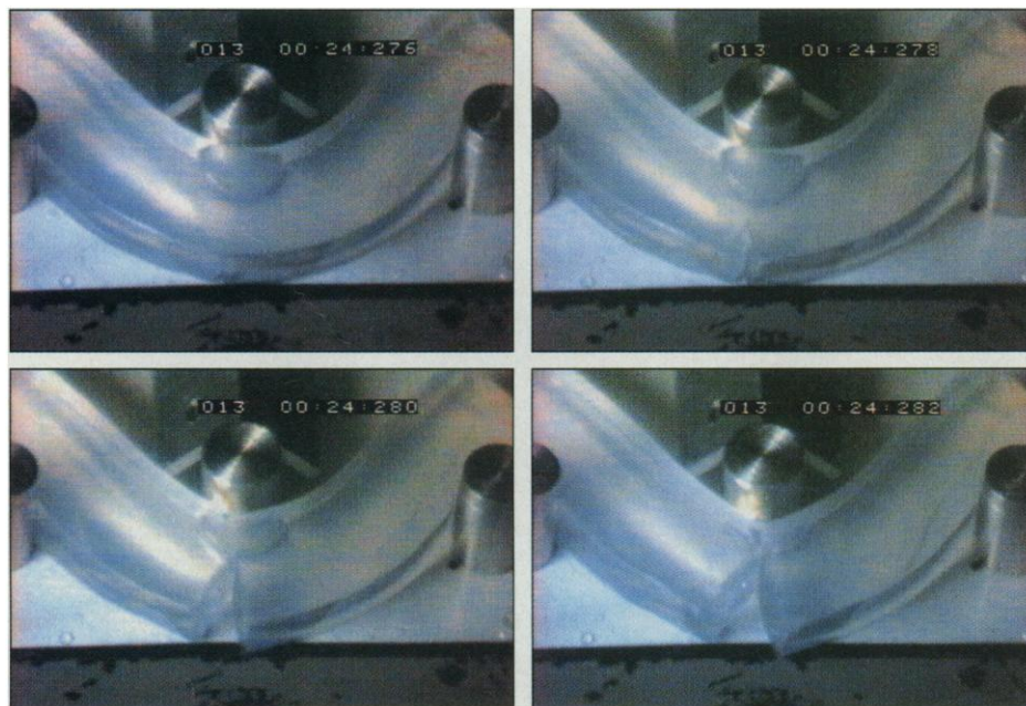
Fig. 2. High-speed photography pictures of the crack propagation. The time between each image is 2 ms.
