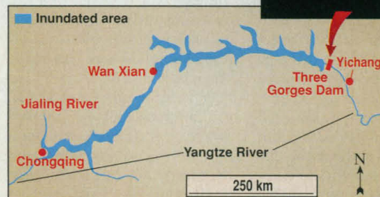
Waterworks. The Three Gorges Dam, the world's largest, will create a 690-kilometer reservoir along a portion of the Yangtze River (inset).
