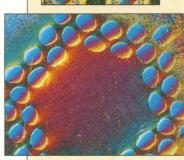
Close encounters. These flea's-eye views of a superconducting wire's 60micrometer niobium strands come from a virtual optical microscope, the latest addition to Molecular Expressions, a Web site run by Michael
