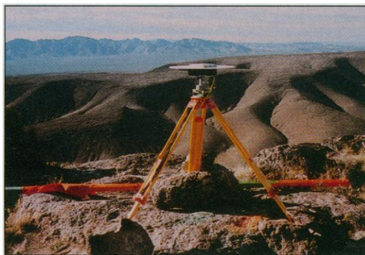
Safe spot? Tripod-mounted GPS receiver measures movement atop Yucca Mountain.
