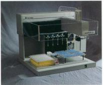
can switch from disposable to washable tips, and transfer samples from any size test tube or vial, to microplates or other labware — all without user intervention. Combine this versatility with a large deck capacity and a bar code reader that can read 256 tubes in 90
