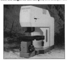
sample, with no need for time-consuming sample preparation. The InspectIR connects to the external beam of any FT-IR spectrometer. It can greatly simplify the analysis of polymers, pharmaceuticals, coated materials, rubber, contaminants, fibers, paper, and forensic samples. Spectra-Tech. For information call 203-926-8998 or circle 145 on the Reader Service Card.
