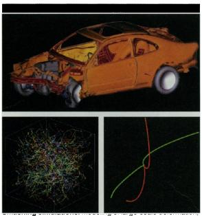
such as in a car crash (**top**, courtesy of Daimler-Benz AG), requires equations that describe the response of a material to an applied load. In the near future, one may be able to obtain such equations from discrete dislocation simulations (**bottom**, **left**, courtesy of B. Devincre CNRS/ONERA); these, in turn, require atomistic input on dislocation core structure, cross slip, and dislocation intersection (**bottom**, **right**).
