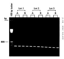
Ready-To-Go RT-PCR Beads mean high reproducibility. A 450 bp fragment from the mouse mitotic checkpoint regulator gene was amplified by two researchers (A and B) using three batches of beads.
