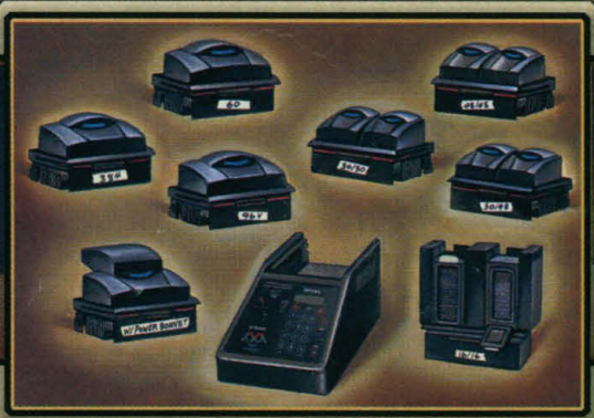
The Tetrad fits four Alpha heads, for up to 8 independent blocks or 1536 reactions
