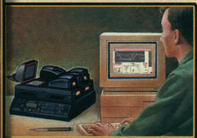
The Tetrad fits four Alpha heads, for up to 8 independent blocks or 1536 reactions
