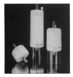
mentation broths, and other solutions and fluids. They make use of two layers of microporous, hydrophilic PES membranes heat-sealed inside a polypropylene housing. This gives researchers a high flow-rate filter capsule with inherently low proteinbinding membranes and low levels of extractables. The filter capsules can be used with a vacuum filtration apparatus, peristaltic pump, or pressurized fluid reservoir. Whatman. For information call 888-WHATMAN or circle 147 on the Reader Service Card.
