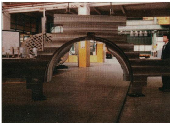
Clamping down. Steel "C-clamps" like this one would brace Ignitor's magnetic-field coils against large stresses.
