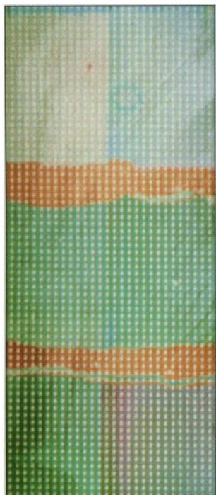
Quick study. Portion of the Berkeley Lab’s combinatorial device array. Each device is about 50 micrometers across.
