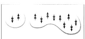
Electrons in boxes. (Left) Schematic illustration of two electrons in a 2D circular quantum dot (quantum dot helium). In the ground state, the spins are oppositely oriented, but in the excited state, they can be in the same direction (triplet state) or in opposite directions (singlet state). (**Right**) Schematic of many electrons in an irregularly shaped 2D quantum dot. The states are expected to be complex, and the ground state may have a net spin polarization.
