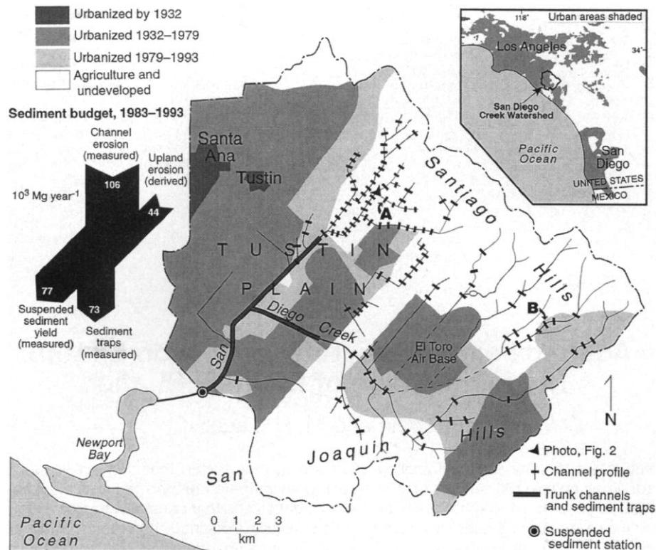
**Fig. 1.** San Diego Creek, showing the earthen stream channel network and the expansion of urban land, 1932–93. Paved channels and channels lying upstream from reservoirs were not included in the study. The cross-sectional channel profiles shown are those remaining in 1993. Sediment yield is that measured at the station plus accretion in the trunk channels and sediment traps. Inset is the sediment budget (balance). A and B indicate the profiles shown in Fig. 3.
