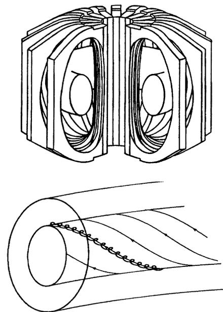
Fig. 1. Tokamak design and typical particle orbit.
