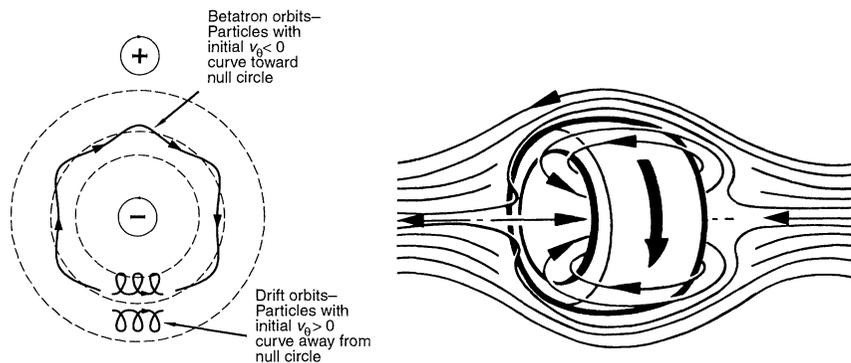
Fig. 2. Field-reversed configuration with typical particle orbits.
