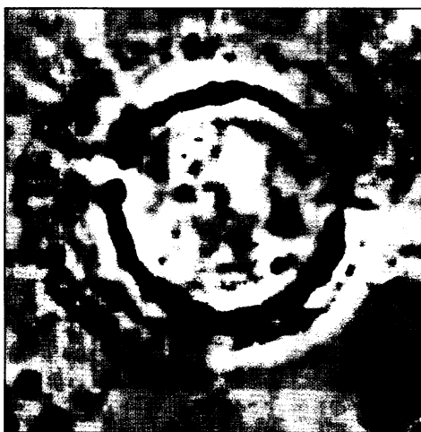
Bull's-eye. Magnetic survey shows ring structure measuring 20 meters across; fainter rings may have been earlier workings.
