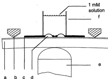
**Fig. 1.** A schematic of the MCB junction with (a) the bending beam, (b) the counter supports, (c) the notched gold wire, (d) the glue contacts, (e) the piezo element, and (f) the glass tube containing the solution.
