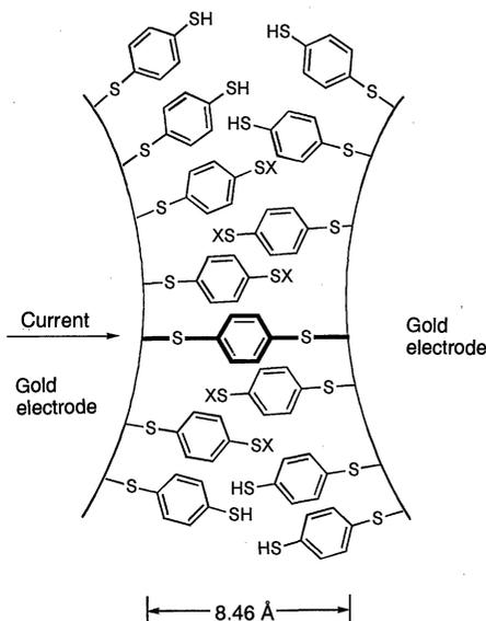
**Fig. 3.** A schematic of a benzene-1,4-dithiolate SAM between proximal gold electrodes formed in an MCB. The thiolate is normally H-terminated after deposition; end groups denoted as X can be either H or Au, with the Au potentially arising from a previous contact/retraction event. These molecules remain nearly perpendicular to the Au surface, making other molecular orientations unlikely (27).
