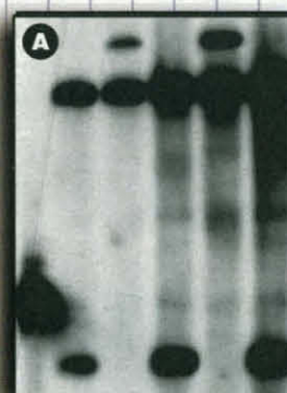
Southern blot, Cosmid DNA digested with Not I and Eco RI, probed with a 1.1kb probe labelled with AlkPhos Direct (A) and digoxigenin (B) (courtesy of Janet Bartels, Yale University).
