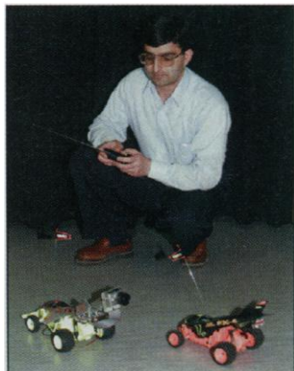
Collision avoider. Toy cars, one equipped with a silicon retina that detects a second car approaching from behind, and designer Alireza Moini.
