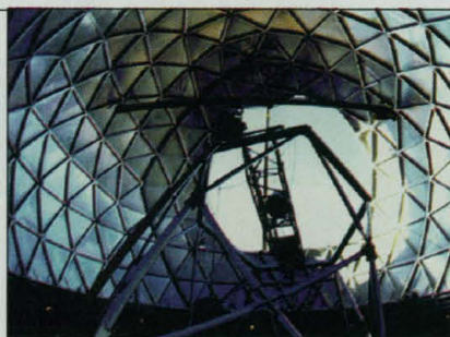
Cost effective. A tracker supports optical instrumentation mounted above the mirror.
