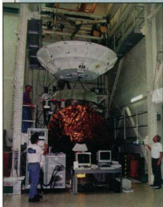
Megamission. The Italian antenna is lowered onto Cassini, with the gold-covered European Huygens probe already attached.
