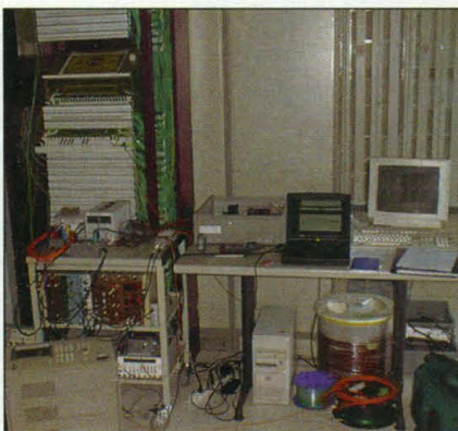
Photons phone home. A photon source (on table), plugged into the Geneva telephone exchange (far left), sends pairs of correlated photons to two nearby villages (map).
