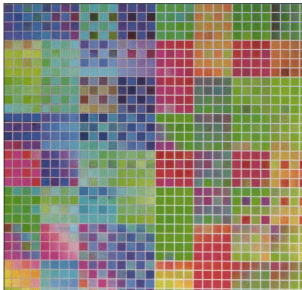
Glowing prospects. An array of different combinations of phosphors being screened for brightness in ultraviolet light.
