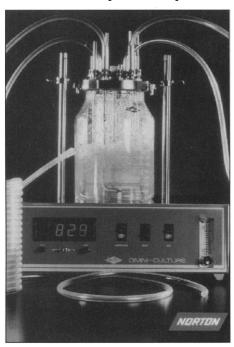
resultant bacterial growth. Its low absorption properties reduce the amount of preservatives and other additives that can migrate into the tubing wall. Adsorption is low as well. The tubing can be cleaned repeatedly by chemical sanitizers and cleaners. Norton Performance Plastics. For information call 800-798-1554 or circle 138 on the reader service card.
