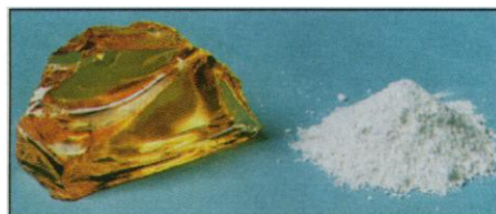
Fig. 1. Bulk tin-based composite oxide (TCO) active material (left). It is a yellowish transparent glass with a density of 3.7 g/cm 3 . Crushing the glass provides a white powder of active material (right) capable of Li insertion for use in the negative electrode of Li-ion rechargeable batteries. The powder typically has a surface area of 0.6 m 2 /g, as measured by the Brunauer, Emmett, and Teller (BET) technique.
