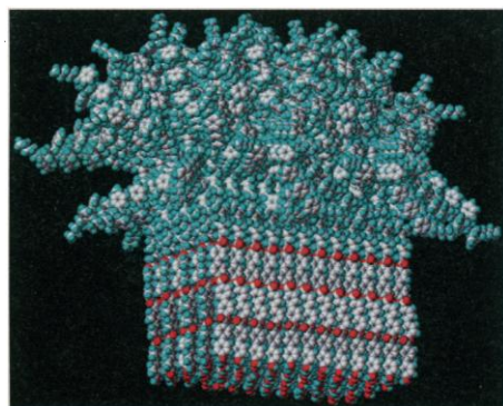
Fig. 6. Molecular model of the supramolecular unit composed of 100 triblock molecules and a molar mass of about 200 kD. Rod segment packing in the mushroom stem is based on electron diffraction data and its rectangular shape on the observation of an oblique superlattice of nanostructures.
